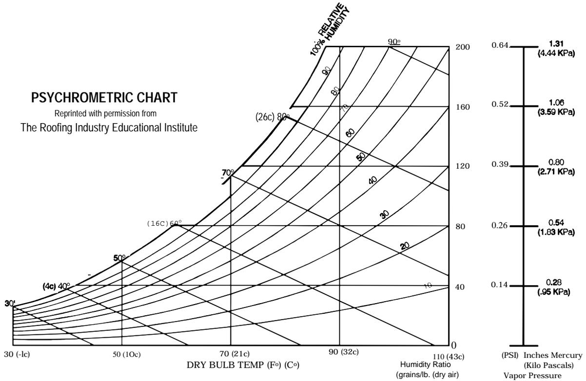
The psychrometric chart is used to determine and correlate the following properties of humid air:
